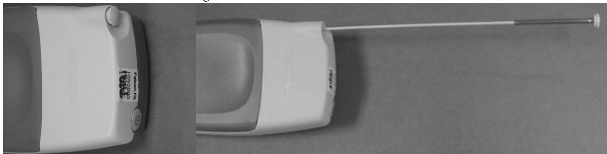
Figure 6: Back of RH-3/RH-3P phone, whip retracted and whip extended
