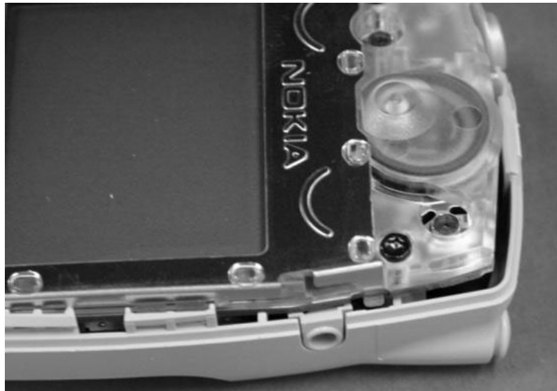
Figure 16: View of display ground clip in assembled phone with A-cover removed
